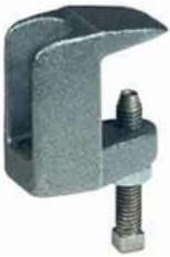
The Top Beam Clamp, MSS (Manufacturers Standardization Society) #58 / 69 Type 19; is used as an upper attachment for many hanger assemblies. Top Beam Clamps such as the NPHC Fig 640 Ductile Iron Beam contains a clamp set screw which is to be torque to 5ft (60") lbs. The NPHC Fig 635 Jr. Top Beam Clamp is used for bar joists and according to NPHC Representatives, its torque instructions are the same for the Fig 640 Ductile Iron Beam Clamp (i.e. 5ft (60") lbs torque.
